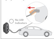
2 - Remove the charging cable from the station..
