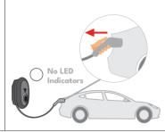
2- Place the charging cable on the socket holder of the station.
